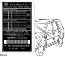
The correct tire pressures are shown on a label attached to the driver's door pillar.
