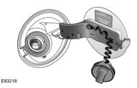
The filler cap is secured to the vehicle by a strap. For your convenience, a holder is provided, on the fuel filler flap, to hook the strap over while refuelling.
